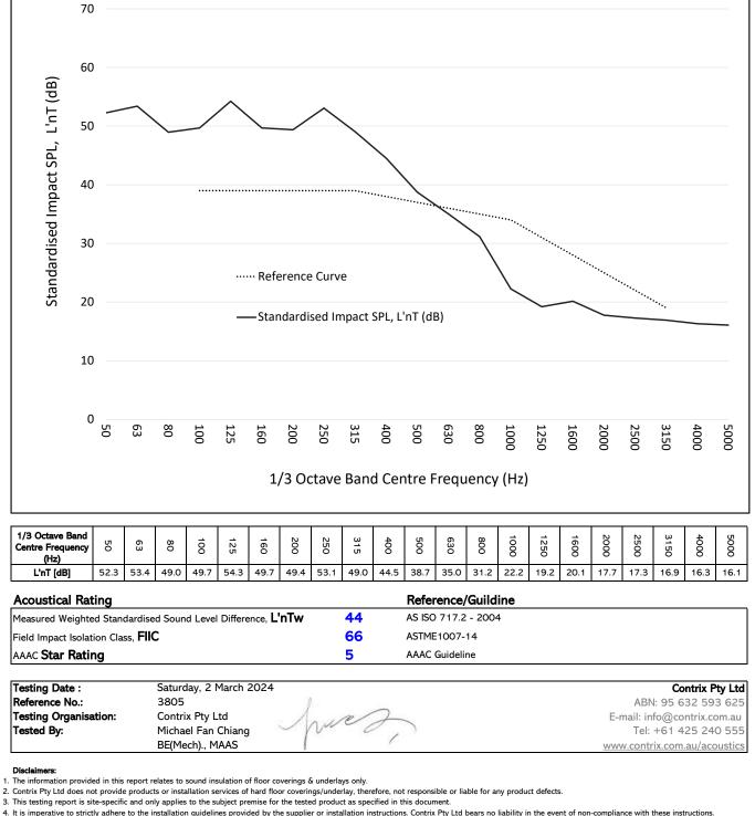
5. The acoustic rating may vary up to 3 rating points depending on the placement of the tapping machine, testing locations within the unit and the junction details between the floorboards/skirting/scotia and
