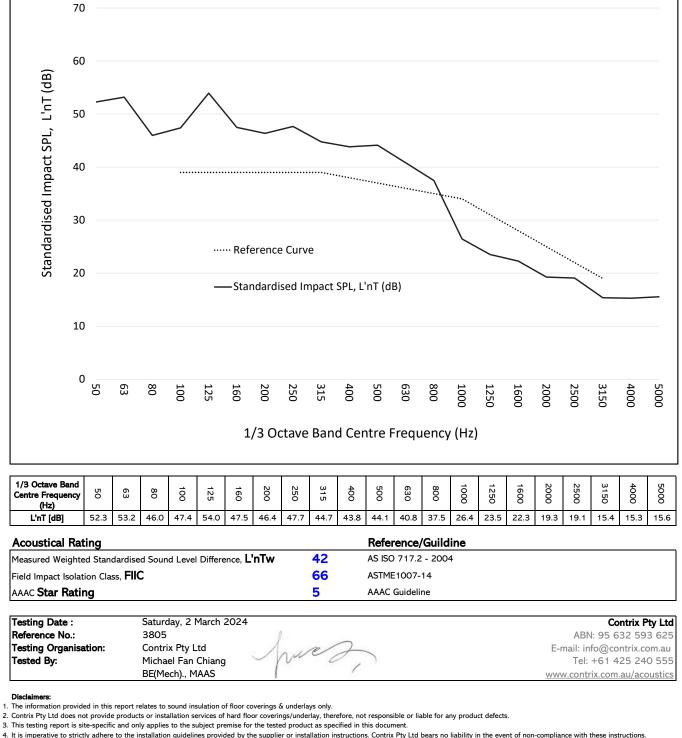
The acoustic rating may vary up to 3 rating points depending on the placement of the tapping machine, testing locations within the unit and the junction details between the floorboards/skirting/scotia and
